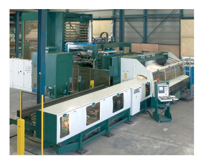
very sophisticated at the same time. "confirmed Aalbers. "When we have to make a production change from sheet to tube, the transfer from the cutting table is made by a mobile carrier with eight centred gripping arms which can pick up tube to a maximum length of 6.5 metres directly from the warehouse stock.
